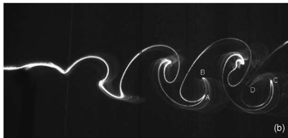
Fig. 15. Spanwise variation of the circulation velocity in an overview picture (a: flow from bottom to top) and in a side view picture (b: flow from left to right) for Re_D = 117 and Ri_D = 0.6 .
